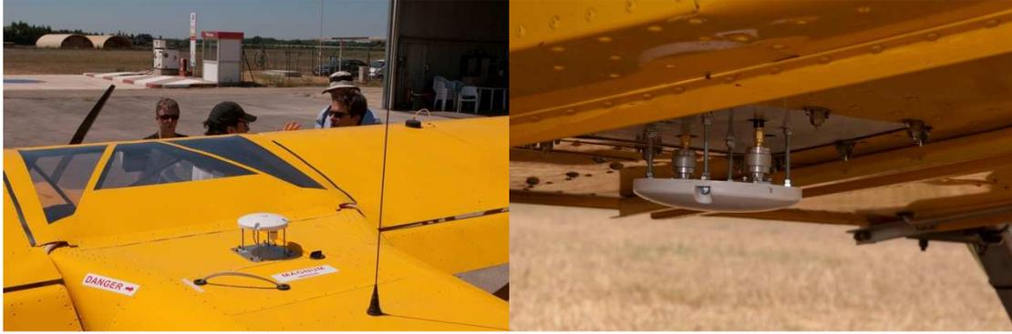
Figure 2- Installed antenna in the top (left) and bottom (right) sides of the ultra light aircraft.
