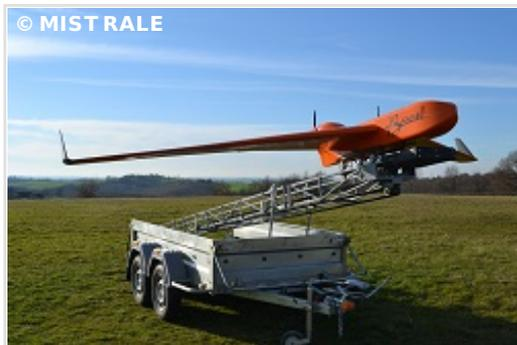
Researchers from the EU-funded MISTRALE project have designed a system which can measure soil moisture from a drone flying at low altitude using GNSS Reflectometry. The system, still a prototype, can produce high-resolution maps of soil moisture by harnessing signals from either the Galileo or GPS global satellite systems. It could help farmers make better decisions about when and where to irrigate and help water managers understand weather events such as flooding and water logging.
